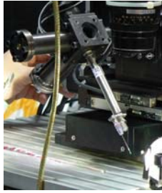
Figure 5: Prototype of micromanipulator with 3 DOF.
