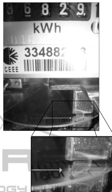
Figure 1: Picture of a tampered meter. There is a stone in the disc.
