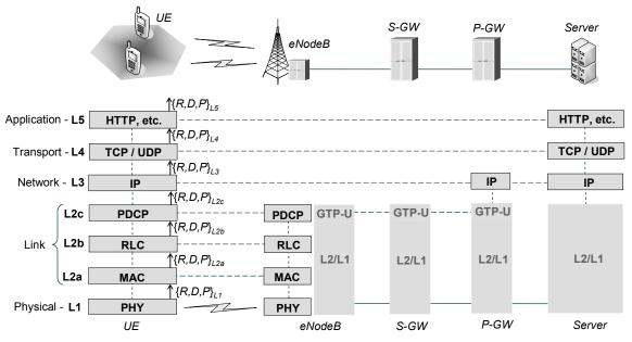
Figure 1: Scenario and protocol stack under analysis.
