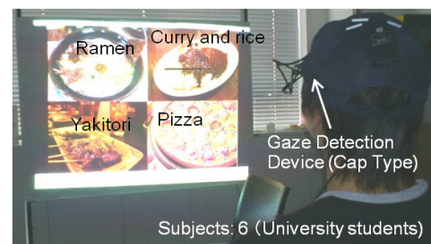
Figure 2: Experimental method of eye catching evaluation.
