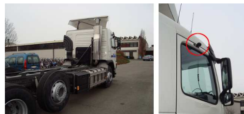
Figure 10: Our test truck (L) with the mounted blind spot camera circled in red (R).
