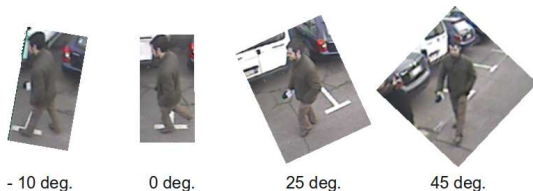
Figure 12: Example one-scale pedestrian detector input images for different rotations.
