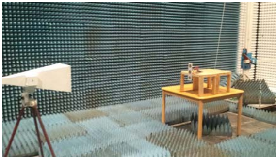
Figure 12: Photograph of intermittent MPT demonstration to a ZigBee end device.
