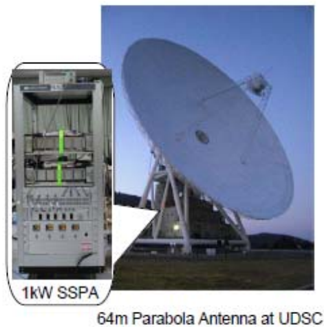
Fig. 1. The kW-class SSPA for the space communication
