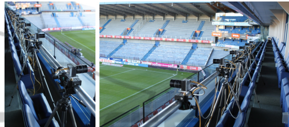
Figure 2: Overview of the camera setup. The setup consists of 8 computer vision cameras with 25mm lenses placed 1 meter apart from each other.
