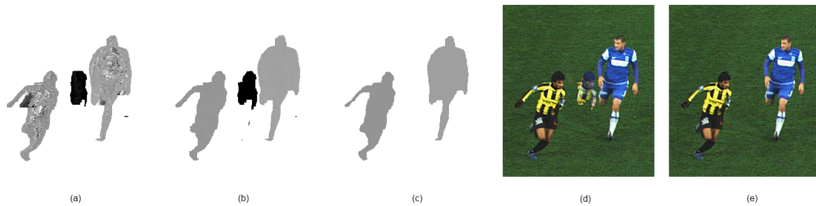
Figure 8: Detail of the method: (a) Depth map of standard plane sweep. (b) Filtered depth map after the depth-selective plane sweep. Not all artifacts are removed. The depth of the artifact differs a lot from the depth of the background. (c) Depth after the depth-selective plane sweep after the removal of the artifact. (d) Result without filtering using the background depth. (e) Result with filtering using the background depth.
