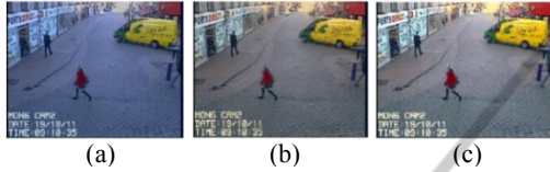
Figure 2: (a) Input video frame. (b) Colour Constancy (c) Enhanced Colour Constancy in HSV domain.
