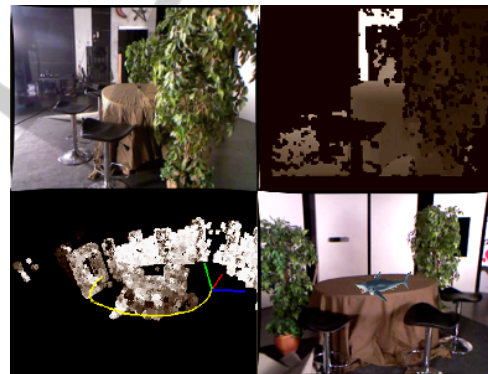
Figure 4: Camera trajectory solved from Kinect input by minimizing the cost function (1). A small shark is rendered into the studio scene.
