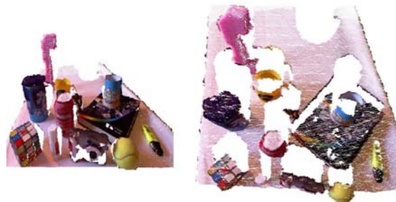
Figure 2: Example of a point cloud from the Kinect camera. Left: view of the visible parts from everyday objects lying on a table. Right: same point cloud from top view, where empty gaps belong to occluded parts.
