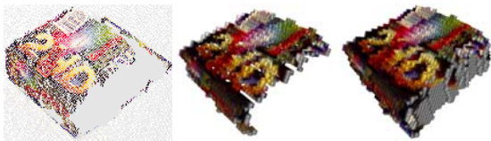
Figure 4: Voxel filling by extrusion. Left: raw point cloud of a box. Middle: voxelized mesh of the raw object cluster. Right: voxelized mesh after extrusion towards the table plane. Gray voxels correspond to unseen parts due to self-occlusions.
