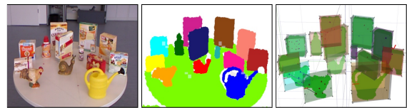
Figure 1: Overview of the approach. (Left) Image of the scene at the first camera pose, (middle) tentative object candidates, or 3D blobs, are identified after scene segmentation, (right) independent- and ego-motion are estimated from the first to the second pose.
