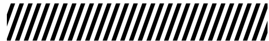
Figure 7: For the desktop setting described in Section 4, the optimal parallax barrier has lines, which are 1.1828mm thick. The lines have a distance of 2.3651mm to each other (measured from medial axis to medial axis) and are rotated by 19.7^\circ .
