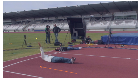
Figure 3: Tracking of the ball to determine the image points needed for the calibration process.
