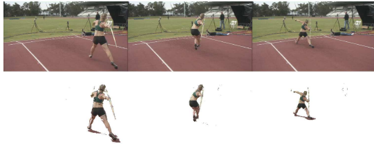
Figure 5: A KDE-based BG segmentation results in one of our outdoors testing trials (Javelin).
