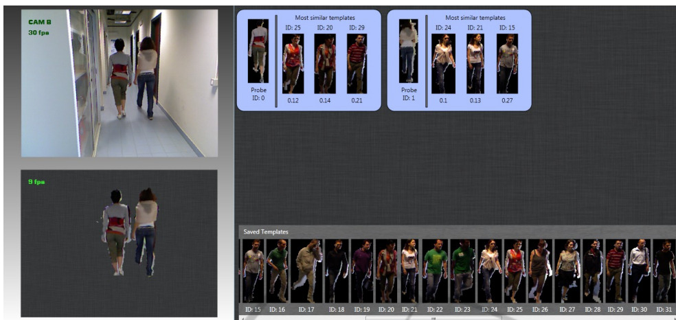
Figure 2: Screenshot of the main view of the prototype GUI, showing images coming from one camera. The user can run many of these views to check simultaneously different cameras. Left: RGB output (top) and segmentation (bottom). Right: the best frame (i.e., the one with the largest silhouette area), the matching score and the template ID of the three template tracks most similar to the one on the left (top); the current template tracks (bottom).
