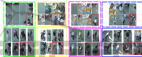
Figure 2: Positive (continuous line) and negative (dotted line) examples gathered from each region. Examples with label errors are surrounded by a red box.
