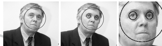
Figure 3: Example of the face detection (left), eyes detection (middle) and the face rotation according to the eyes (right).
