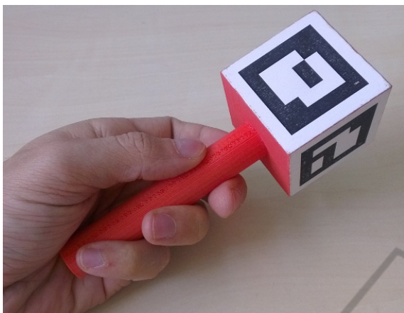
Figure 1: This device is tracked by a computer with a webcam. It is used as a 3D input device for direct manipulation.
