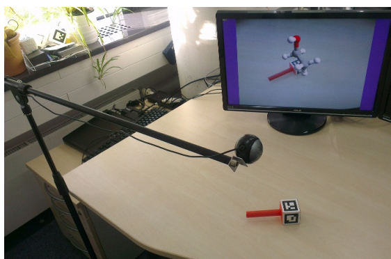
Figure 3: Computer setup for the ACR application, using a webcam a physical cube on a handle and a monitor. The keyboard that is required to cycle through a set of molecules is not shown.
