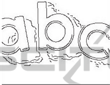
Figure 8: Binary edge image using Deriche operator.
