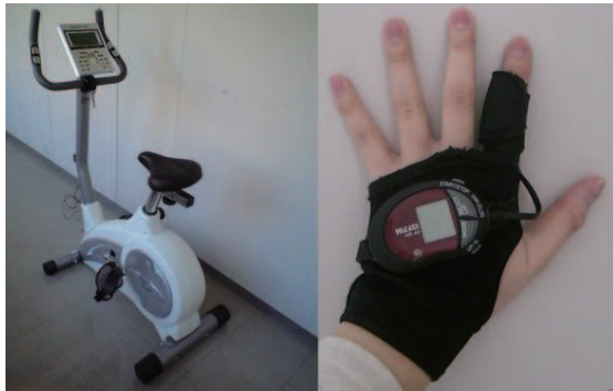
Figure 2: Left: Programmable ergometer, AFB6008. Right: Photoelectric pulsometer, Pulse Coach Neo HR-40.
