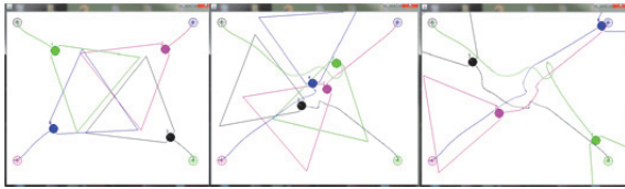
Figure 5: Simulation 1: Collision avoidance simulation with four robots.
