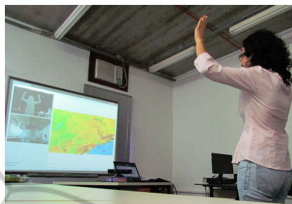
Figure 7: User's interaction recorded by cameras as well as the user's representation and the Terrain Viewer system projected in the screen.
