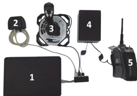
Figure 2: Ground station (1) Computer (2) RF receiver (3) Joystick for assisted teleoperation (4) Duplicate onboard RF-receiver acquisition system (5) Radio control for manual operation.
