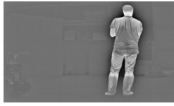
Figure 7: The image shows a clearly visible thermal structure of a person which helps people detection, because more features can be extracted on the person.
