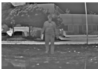
Figure 2: On this thermal image, the person has a very low contrast to the background, because of high temperatures in the surroundings. This makes it impossible to find a fixed temperature threshold to separate person and background reliably.
