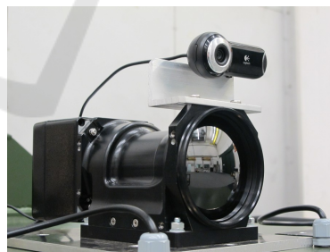
Figure 1: Camera setup. The USB camera is mounted on top of the thermal camera so they both capture images of the same scene.
