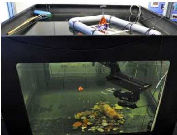
Figure 17: Underwater platform with ARM5E robotic arm used to perform water current tests.
