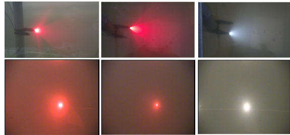
Figure 16: Underwater visibility experimental results on increasing water turbidity.
