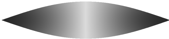
Figure 5: The planar projection of the FoV for the tilting LRF, the gray scale represents the distribution of sampling points, where the black correspond to the highest concentration.
