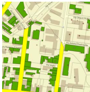
Figure 4: Results of the SPARQL query as a vector data layer on Quantum GIS. The raster data is derived from OpenStreetMap, the green polygons represent buildings, the yellow highlighted sub-layers of the parcel represents the streets. The points return, if clicked, geo-referenced tax information.
