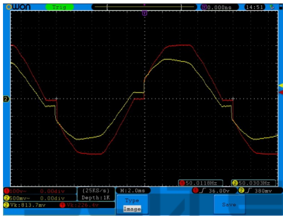
Figure 8: High \Delta I/\Delta t transient causing high RF disturbance.
