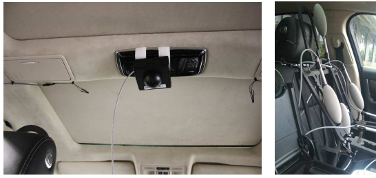
Figure 1: Experimental data gathering. Left: Mean radiant temperature sensor. Right: Upper body of the Flatman thermal manikin.
