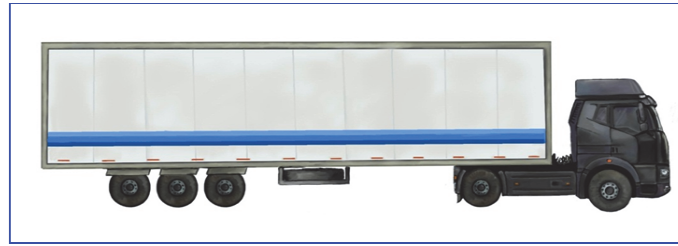
Figure 2: Experimental truck “Volvo FH12” with full load 36900 kg.
