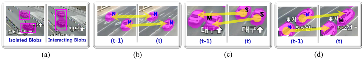
Figure 3: Figures for the blob-level tracking processes: (a) Examples of isolated and interacting moving blobs in a scene. We collect only isolated blobs for the subsequent S3W-pattern modeling because bounding boxes for merged blobs cannot provide accurate vehicle size information as shown in 'Interacting Blobs' figure; (b), (c) and (d) describe blob-matching results in the isolation, split and merging state, respectively. Yellow arrows show matching directions, and letters N , M and S imply that corresponding blobs are in N_{state} , M_{state} and S_{state} .
