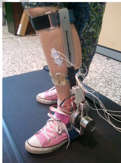
Figure 1: MAFO (motorized ankle foot orthosis), worn by one of the subjects of the study.
