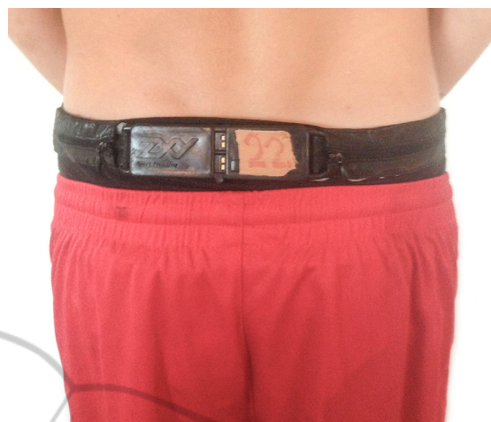
Figure 1: The ZXY Sport Tracking sensor belt.
