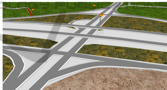
Figure 11: The result of applying the RAV reconstruction algorithm on the interchange in Figure 10.
