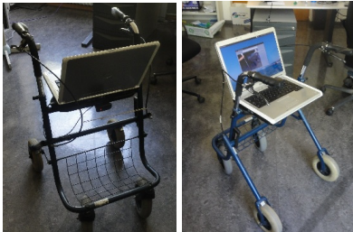
Figure 1: Walker used in the study, equipped with a webcam and computer. It is a typical walker with four wheels, handles with breaks and a seat
