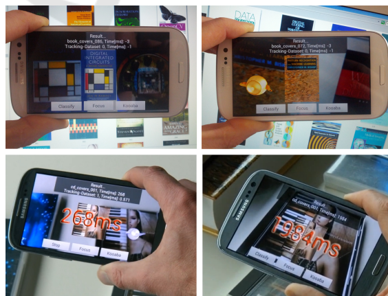
Figure 1: Mobile prototype: top-left: client-side visual search, top-right: tracking and augmenting an image target recognized by client-side visual search, bottom-left: fast switching of tracking datasets with the local pipeline (268 ms); bottom-right: slow recognition using the server-side approach (1984 ms).
