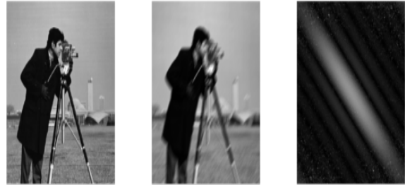
Figure 3: Left: Sample image. Center: simulated camera motion at 45^\circ . Right: Fourier transform of the center image.
