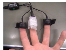
Figure 6: State of attaching an SC sensor and a BVP sensor.
