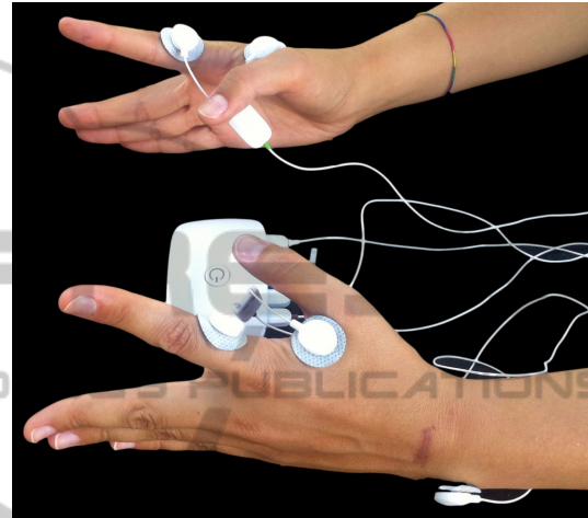
Figure 2: Contralateral acquisitions experimental setup: Bioplux research device, placement of two EMG sensors and ground.
