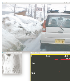
Figure 20: The result of a real road scene 2 (Front camera).
