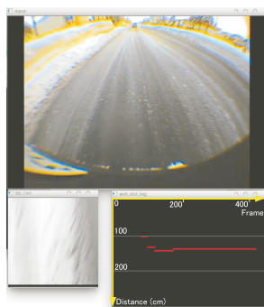
Figure 13: The result of a real road scene 1(Backup camera).
