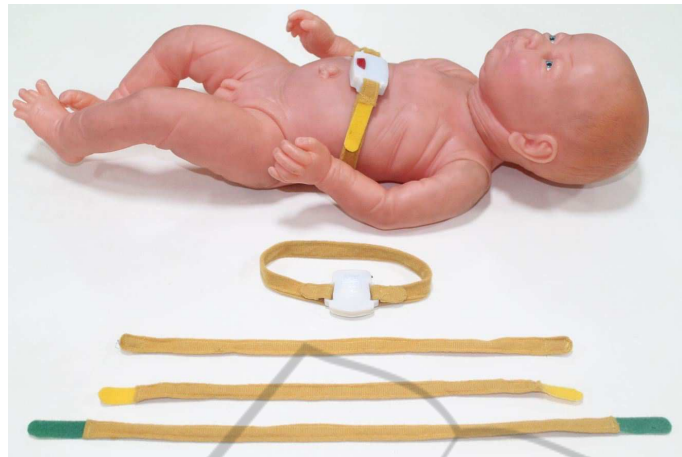
Figure 6: Prototyped temperature sensor with belts.
