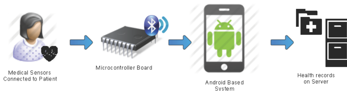
Figure 1: End-to-End Data Flow of the mDROID System.
