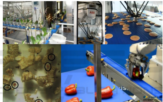
Figure 1: Examples of industrial object categorization applications: robot picking and object counting of natural products. [checking flower quality, picking pancakes, counting micro-organisms, picking peppers]
