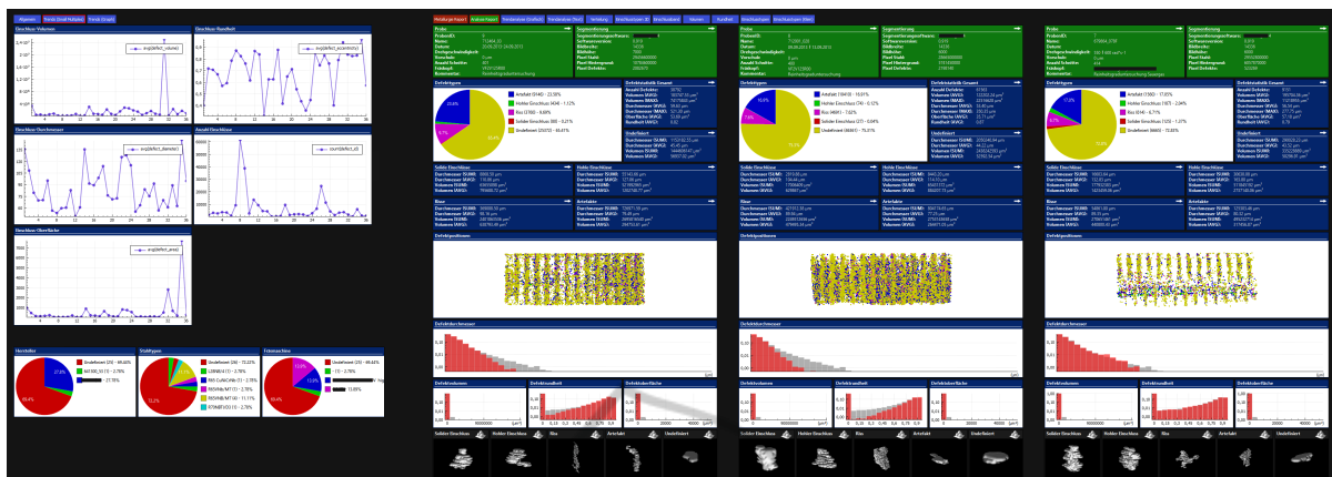
Figure 2: This screenshot shows the level of traversal set to samples. The samples of the current data tree are visualized. Each sample is presented in multiple views consisting of various visualization types and data from different hierarchical levels (context+detail). Level overview visualizations are positioned on the left side. By scrolling further to the right, more samples can be seen.
