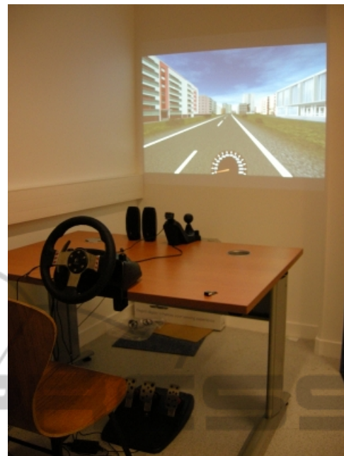
Figure 1: Scene setting of the experiment in simulated driving environment.
