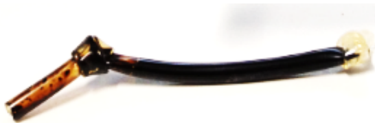
Figure 8: Plastic sheath of 3mm filled with ferrofluid.
