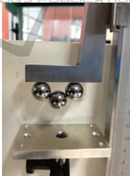
Figure 6: The 3 magnets in the “loop” configuration.
