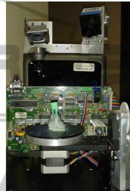
Figure 1: Optical scanner during the acquisition process of a tooth template.
