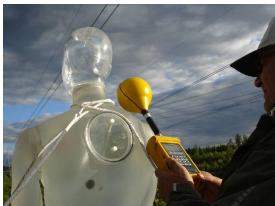
Figure 3: An example of magnetic field measurement.
