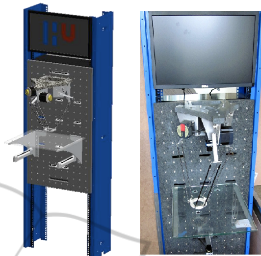
Figure 2: On the left of an equiplet with a deltarobot and glassplate working area module attached. Right a real equiplet prototype with a deltraobot module and a glassplate working area that is used to observe with a computer vision system to localize parts.
