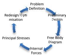
Figure 3: Design Loop for a gantry beam using Solid Mechanics fundamentals.
